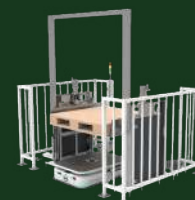
Pallet Lifting Station
